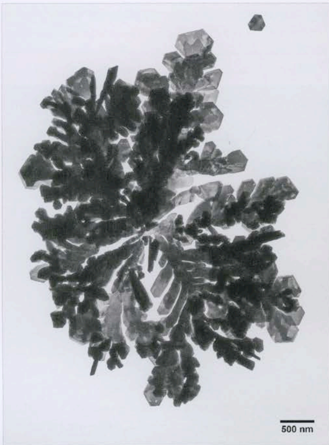
Student: Lindsay Quandt, RIT, Imaging and Photographic Technology. Photograph by Richard Hailstone. Host/Client: Undergraduate Research Assistant for Dr. Grover Schwartzlander, RIT College of Imaging Science. Assignment: Develop ways to chemically induce the formation of silver nanorods along stretched polarizing polyvinyl alcohol (PVA) using transmission electron microscope (TEM) imaging to evaluate results. Pictured: A silver structure formed from silver nitrate and sodium diphenylamin-4-sulfonate in PVA, August 2012
