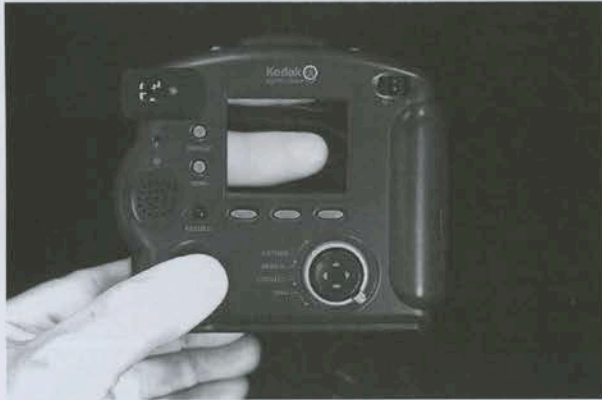
Figure 5 Liquid crystal display (LCD). The LCD preview is an excellent tool to assess proper exposure, correct focus, evaluate composition and perspective, and confirm the correct color
