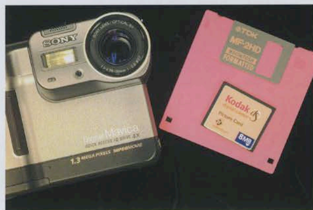
Figure 10 Mavica and disk. Sony adopted a different storage medium approach than other brands for a less equipment-dependent approach. The Mavica uses the standard floppy disk rather than newer unique memory cards. Included in this picture is the Kodak Compact Flash disk for reference to a compact card
